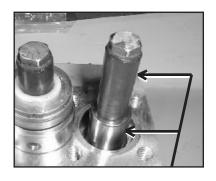
9) Check surfaces of plunger pipe (16B).
